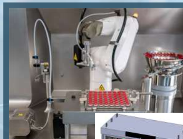
Semi-automatic robot filling line at Supply Center Berkeley and future Adherent Cell Therapy using Smart Robotics
