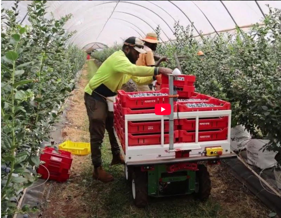
Burro (deployed in Australia) for autonomous carts used for harvest assist, spraying, mowing, and material hauling.
